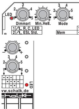
The LED is lit in the On state. In the Off state it blinks intermittently if the dimming mode or the operating mode has been changed. If a fault occurs, it displays a fault code.
